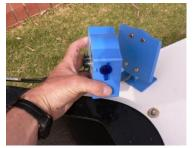
Plug microphone into 'Mic' socket. Press  $\bigcirc$  button to turn unit On. It will briefly display '**ON**' and then charge level eg '**C56**'. It will give a short beep through speakers – this lets you know the speakers are connected. It will then display stroke rating if seat sensor is activated, eg '**25.8**' means 25.8 strokes per minute. If there is no signal from seat sensor for 12 seconds '---' will be displayed.
