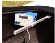
to rate. If you want to display time continuously, press the [Display] button – this toggles display between rate and time. The example display represents 3 minutes and 59 seconds.
